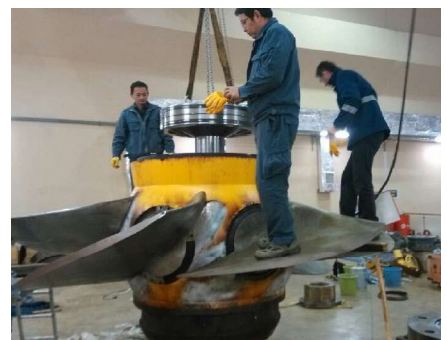
Runner checking for Kaplan turbine
