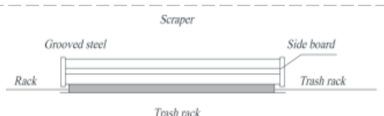
Fig. 3 The comb-scraper for cleaning up trash rack
